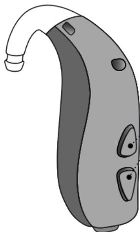
• Apply a very long press (4 seconds) to either end of the button to mute the hearing aid.
