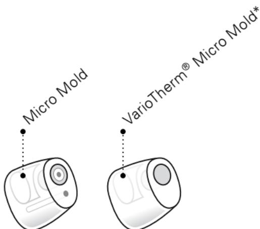
Customized earpieces have a white wax filter attached to the sound opening. ProWax is the filter type to be used with these earpieces. To replace the ProWax filter, see section “Replace ProWax filter”.
